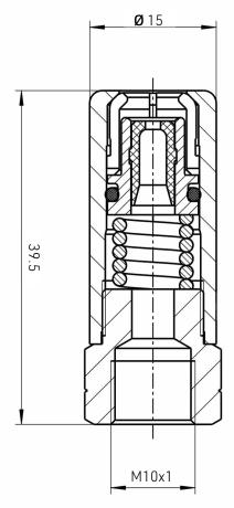
Special Four-Jaw Coupler; heavy-duty, high-pressure version, for reliable, efficient grease transfer from the Amtec Handpumps to the Amtec F-Nipple mounted in the Amtec F-Type Hydraulic Nuts.
