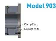
Circular knife I.D. equals the clamp ring I.D. The knife is bolted against the face of the clamp ring.
