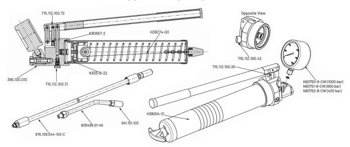
112.100.200-XXX Rod Type Handpump Parts Breakdown
