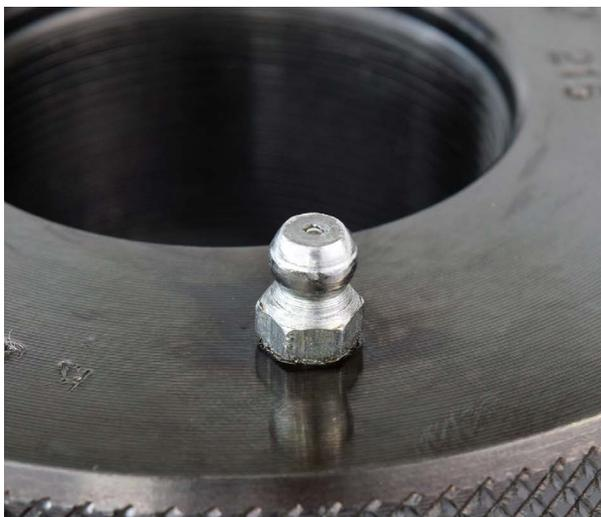
8. Apply a handpump to the nipple and then pump grease through the nut until the grease exiting the open filling screw hole is clean and free from air bubbles. Remove the handpump.
